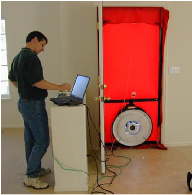
Figure 1: Blower Door Test
